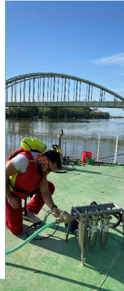
Figure. Microplastic sampling using net device and suction pump on Argus ship – Tisza River (Titel, RS)
